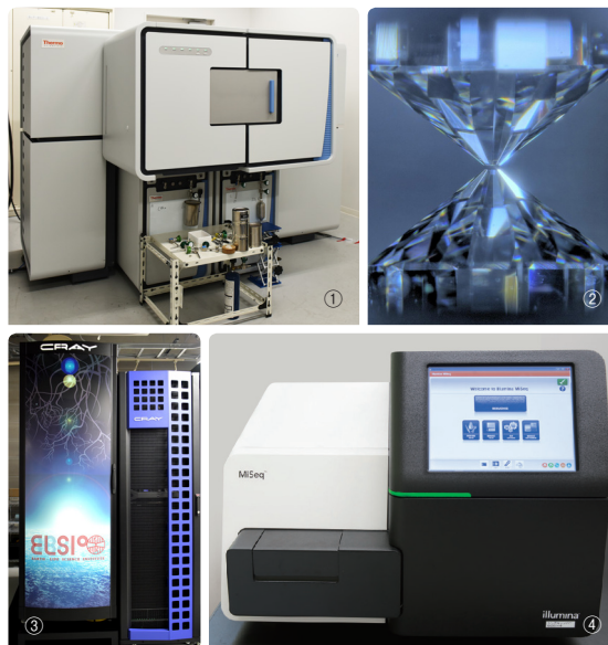
① High Resolution Isotope Ratio Mass Spectrometer (Thermo Scientific™ 253 Ultra™) enables the measurement of molecules that consist of multiple heavy isotopes. ② Comprised of natural diamonds, the Diamond Anvil Cell is a device that generates ultra-high pressure. ③ Cray XC30™ Supercomputer is used to investigate a variety of research. ④ Next Generation Sequencer (NGS) analyses genomes using a massive parallel sequencer.
